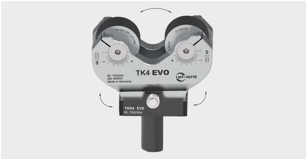
Figure 14: Checking the pendular play of the rolling head in the holder
